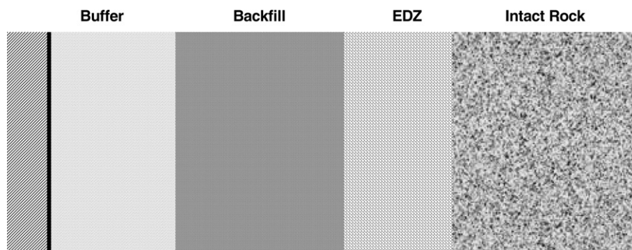
Fig. 6. Schematic representation of the series of 1-dimensional mass-transport barriers used in the model to simulate the various engineered and natural barriers.
